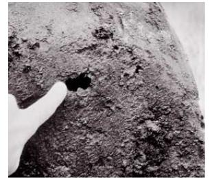
Old buried fuel tanks often rust through and leak contents directly into the soil.
